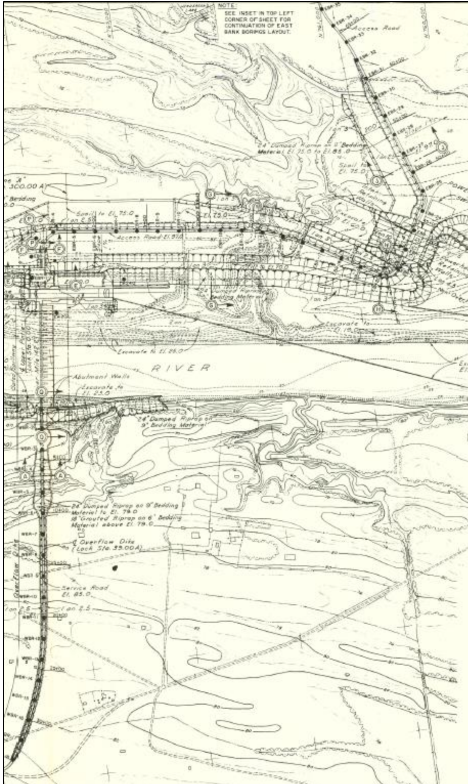
Figure G-1: Geotechnical investigation boring approximate locations for the left and right embankments used for the feasibility level geotechnical analysis
